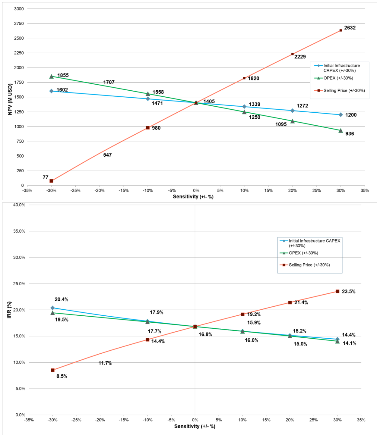
Figure 4 – Sensitivity to post-tax NPV8 and IRR (Base Case) based on changes in FOB Iron Ore Price
